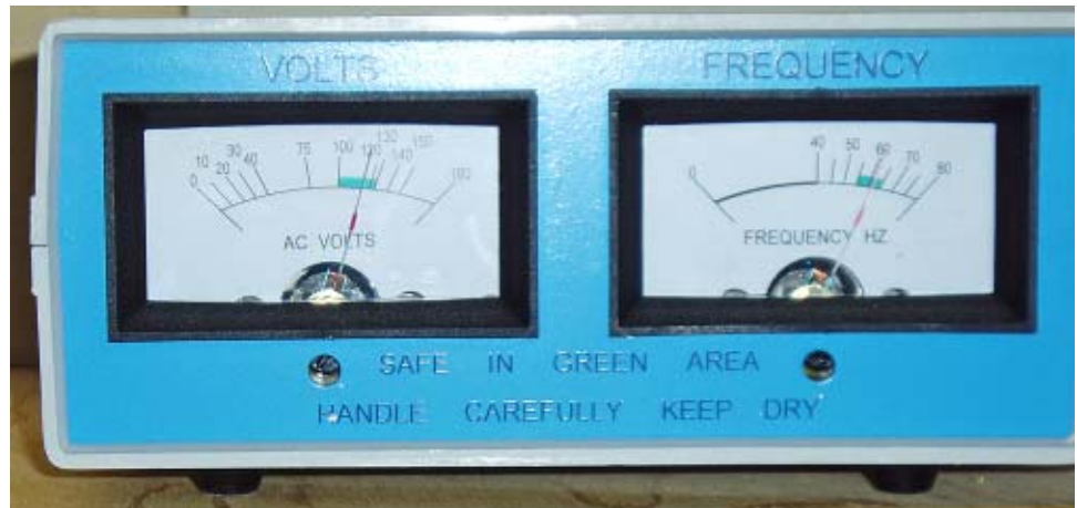
It is very important to monitor the voltage and frequency output of generators. This inexpensive unit plugs into a 115 volt receptacle for quick and easy on site adjustments, but does not allow for remote monitoring functionality.
