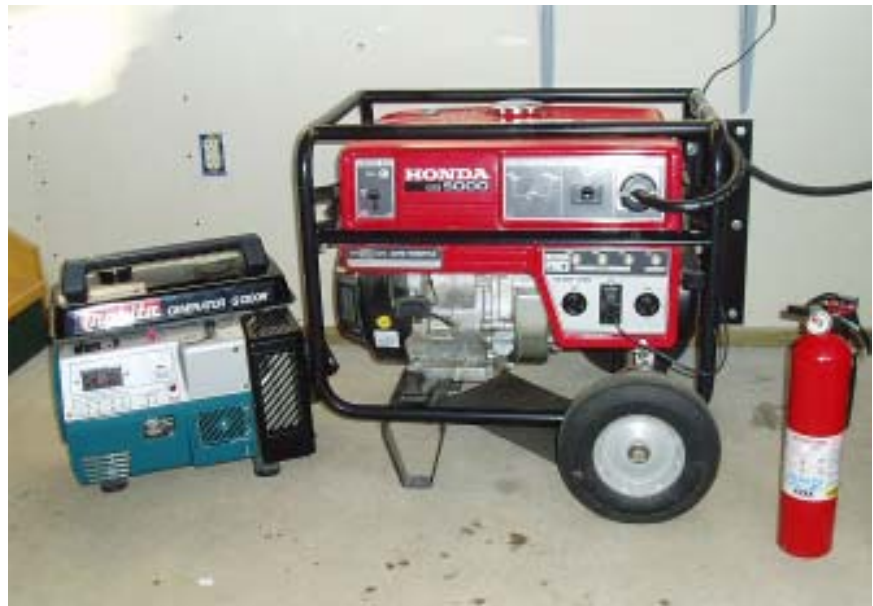
The Makita G1300R on the left is a 1.3kW unit and is considered a portable model. The Honda EB5000 on the right is a 5kW unit. While still portable, it weighs nearly 200 lbs., and is more typically classified as an “industrial” generator.
